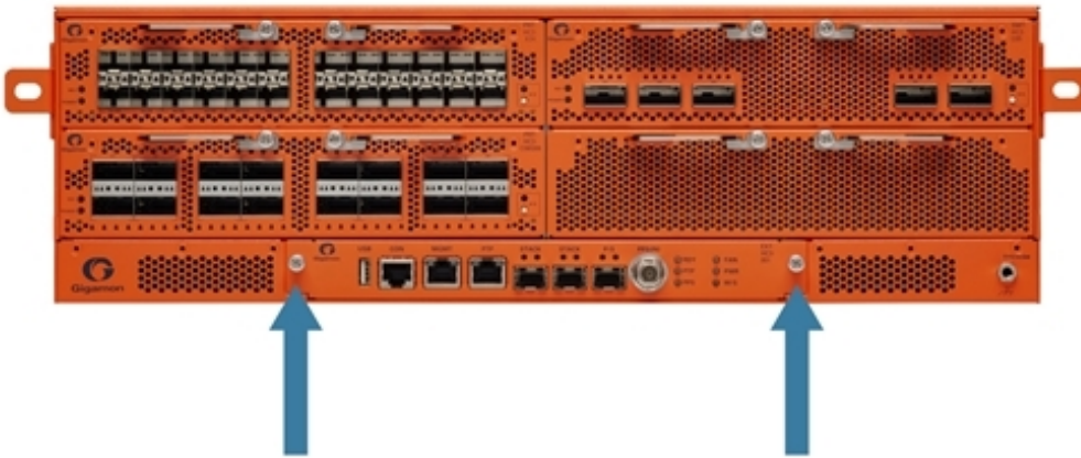
Figure 15 Extension Board Screw Location on GigaVUE-HC3 Front
